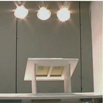
A bank of infrared lamps is arranged to shine on test materials mounted at an angle approximating a roof exposure.
