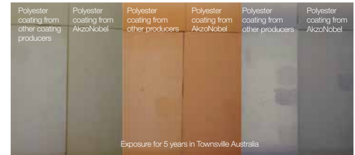
Figure above: Three sample groups of exposed panels; the small one above is the original color and the below is the color following exposure. The three groups of samples are all polyester coating systems. According to the result of exposure in Townsville Australia, the sample on the right is superior to the sample on the left. It shows that the selection of resin and pigment type is very critical to the product performance.
