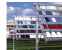
Natural exposure rack
