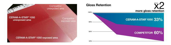
**Color Fade:** CERAM-A-STAR 1050 retained an average  $\Delta E$  of 1.6. **Competitor panels faded 1.5 times more** than CERAM-A-STAR 1050. This means that projects stay looking the original color for longer.
